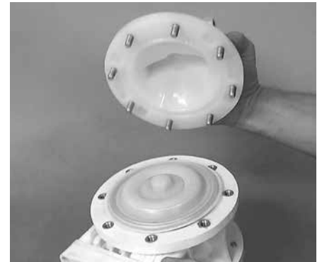
Step 8. Figure 8 The liquid chamber should be removed to expose the diaphragm and outer piston. Rotate center section and remove the opposite liquid chamber.
