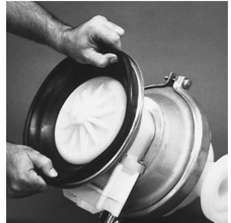
Step 11. Figure 11 Using an adjustable wrench, or by rotating the diaphragm by hand, remove the diaphragm assembly.
