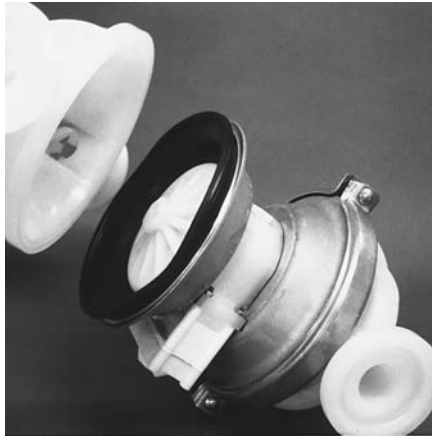
Step 10. Figure 10 Lift liquid chamber away from center section to expose diaphragm and outer piston.
